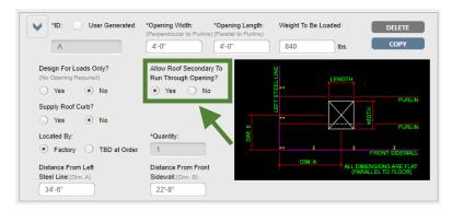
The first detail to look at is the weight of your RTU. Kirby Building Systems guidance requires that any RTU weighing more than 1,000 lbs. should have independent framing members. These members are usually built-up or hot rolled beams used to support the heavier RTU loads. This type of framing requires purlins to be cut, so there is little benefit for allowing purlins to run through the opening.
