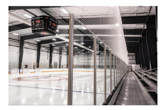
The facility features Kirby's KirbyLok Mechanical Roof System in galvalume, and the DM40 Insulated Metal Panel Wall System. Kirby provided clear span designs of 140' for the indoor fieldhouse and 115' for the ice rink section.
