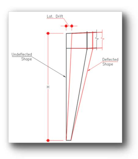
Figure 1 - Frame Lateral Drift (sidesway)
