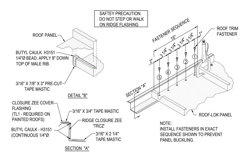
CAULKING AT THE PANEL SIDELAPS AS SHOWN IN DETAIL "B" ABOVE IS CRITICAL TO INSURE WEATHERTIGHTNESS. CLAMP VERTICAL SEAM OF PANEL TO INSURE MASTIC ENGAGEMENT AND TO MAINTAIN MODULARITY UNTIL FASTENERS ARE INSTALLED. POSITION RIDGE CLOSURE ZEE (TRCZ) ONTO PANEL ENDS HOLDING IN PLACE WITH C-CLAMPS. ATTACH WITH ROOF TRIM FASTENERS AS SHOWN. COMPLETE SEAM WITH HAND SEAMER.
