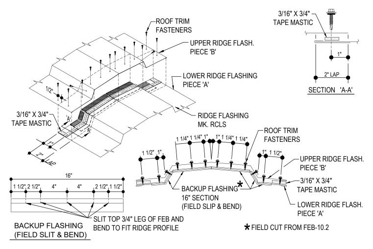
NOTE: HOLES MUST BE PRE-DRILLED AT RIDGE FLASGING PRIOR TO APPLYING MASTIC. TEMPORARILY LAP PIECE "B" OVER PIECE "A" AND PRE DRILL THE REQUIRED NUMBER OF 1/4" Ø HOLES THROUGH BOTH PIECES OF RIDGE FLASHING BUT NOT 'FEB' BACKUP FLASHING. SLIDE PIECE "B" BACK AND APPLY TAPE MASTIC AND BACKUP FLASHING ON PIECE "A" AS SHOWN. LAP PIECE "B" OVER PIECE "A" BEING CAREFUL TO ALIGN HOLES. INSTALL ROOF FASTENERS AS SHOWN. CONTINUE PROCESS AT EACH RIDGE FLASHING END LAP AND ALONG THE RIDGE.
