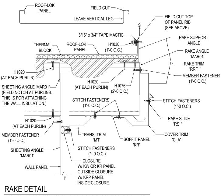
STARTING DETAIL, ON MODULE, RAKE EXT., W/ KR SOFFIT, ROOF SLOPE < 2:12
