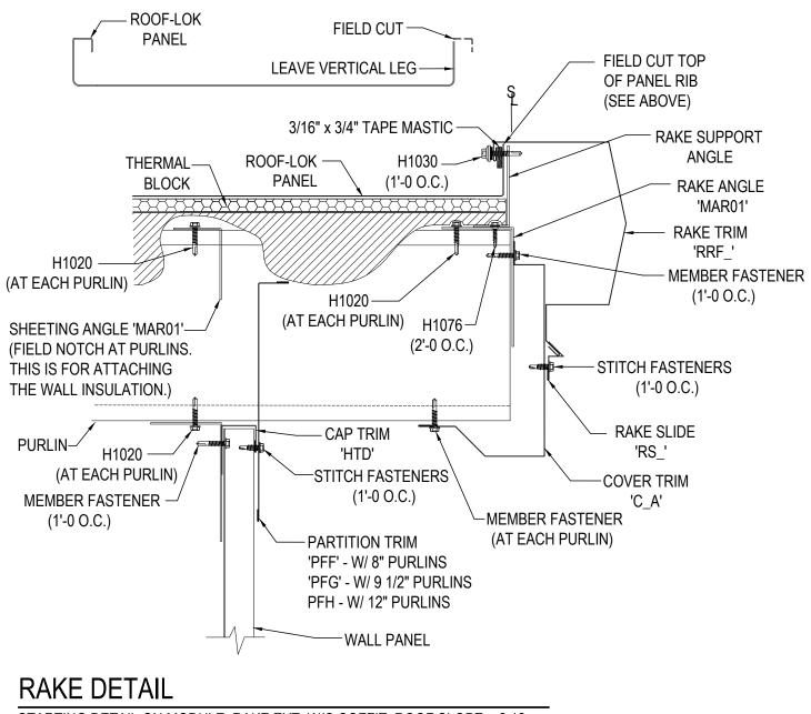
STARTING DETAIL ON MODULE, RAKE EXT, W/O SOFFIT, ROOF SLOPE > 2:12
