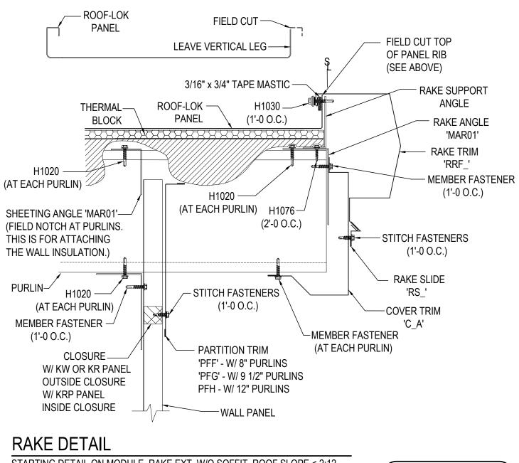
STARTING DETAIL ON MODULE, RAKE EXT., W/O SOFFIT, ROOF SLOPE < 2:12
