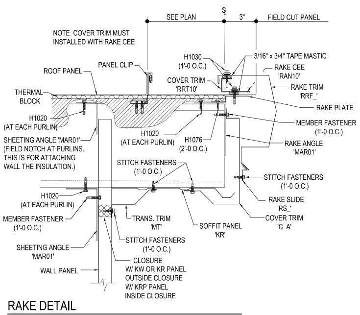
STARTING DETAIL OFF MODULE, RAKE EXT., W/ KR SOFFIT, ROOF SLOPE < 2:12
