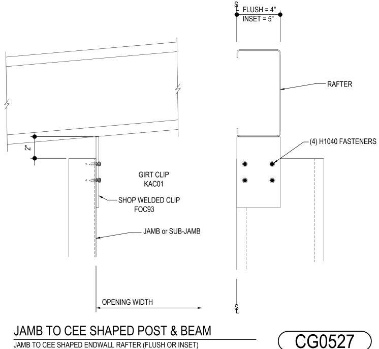
JAMB TO CEE SHAPED ENDWALL RAFTER (FLUSH OR INSET) REFERENCE A00010 FOR WASHER REQUIREMENTS
