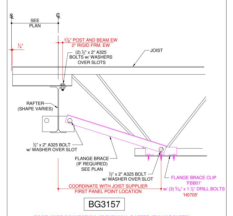
ROOF JOIST CONNECTION AT ENDWALL RAFTER (FULLY BOLTED)
